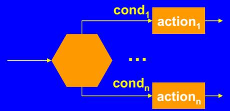
Therefore every synchronous UML activity diagram can be viewed as a synchronous multi-agent ASM whose agents are control state ASMs with rules representing alternating branching and action nodes
